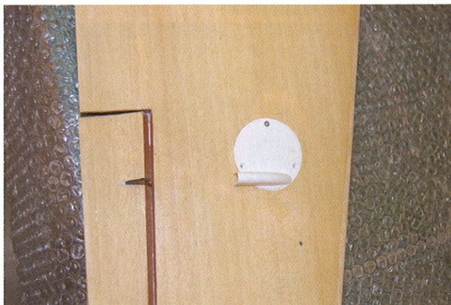
Ailerons fitted into wing and neat servo cover
