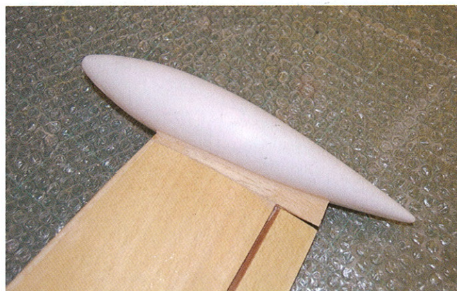
Wingtip tank secured to wing with glue
