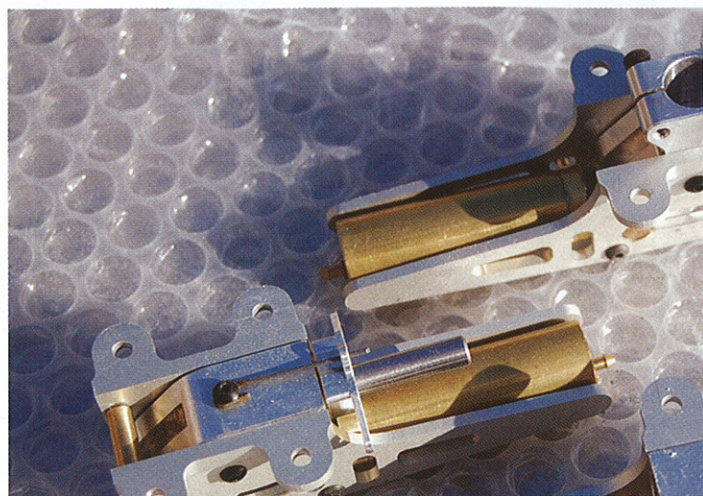
Left: MAP air up air down retract units, not units often seen in the UK
