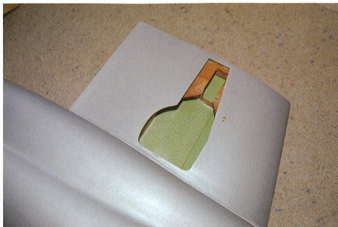
Wing stubs hold the retract mounting plates
