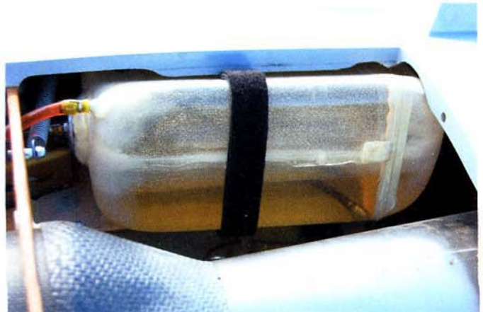
Method of securing tanks using straps
